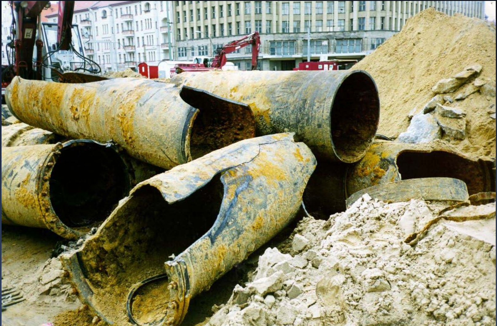
Pipe burst: aged water infrastructure
